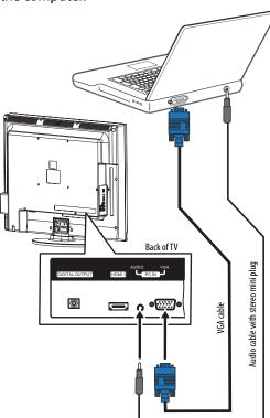
3 Connect an audio cable with stereo mini plug (not provided) to the PC IN AUDIO jack on the back of your TV and to the LINE OUT or AUDIO OUT jack on the computer.
